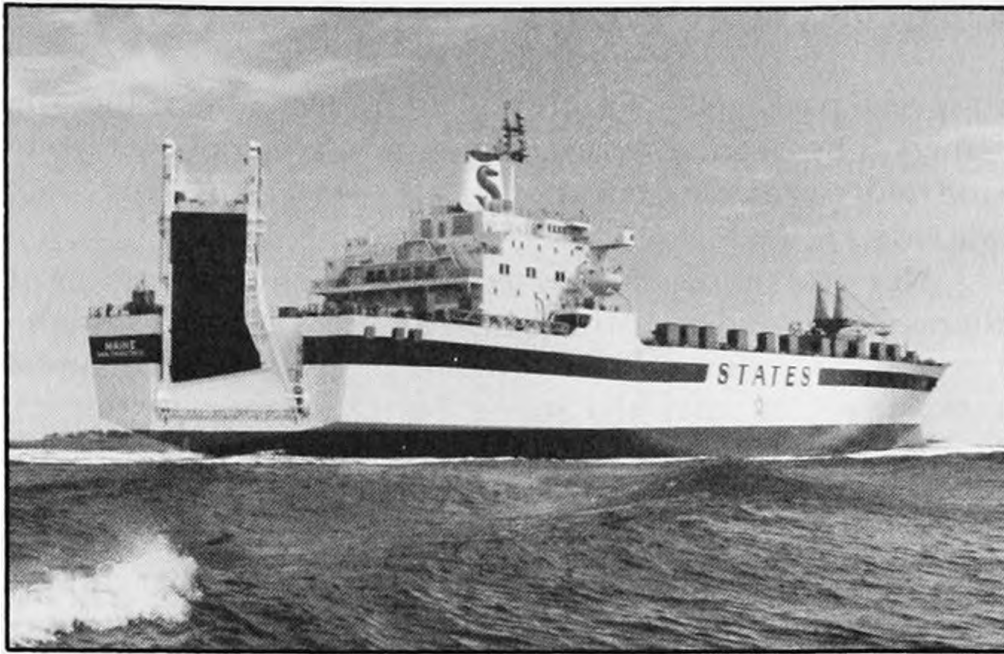
The Bath Iron Works "Ro-Ro" Maine is the lead ship in a class of four such vessels. The freighter, built with a large stern ramp to service ports with underdeveloped facilities all over the world, was launched in late 1975. Courtesy Bath Iron Works.
